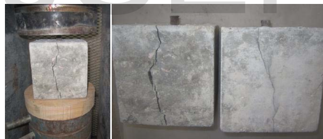
Figure 5. Modes of failure of concrete specimens after the bond strength test.
